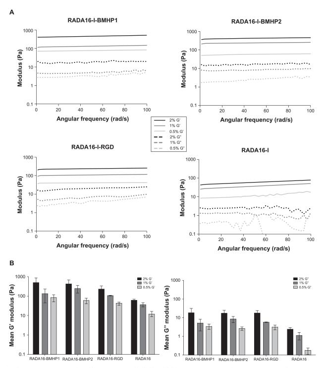
Figure 9 Rheological characterization of each SAP at concentrations of 0.5%, 1%, and 2%. A frequency sweep test was performed on the assembled scaffold, between 1 and 100 rad/s. A) Elastic shear modulus G' and viscous shear modulus G' values for each SAP, along the frequency sweep test. B) Mean G' and G' values for each SAP, calculated from data presented on A.
