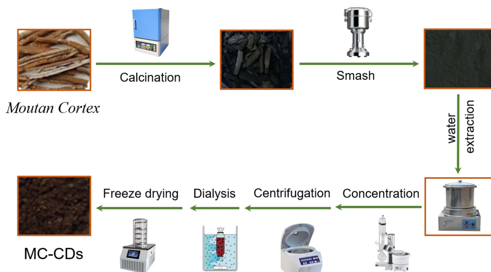
Figure 1 Preparation scheme of Moutan Cortex -Carbon dots (MC-CDs).
