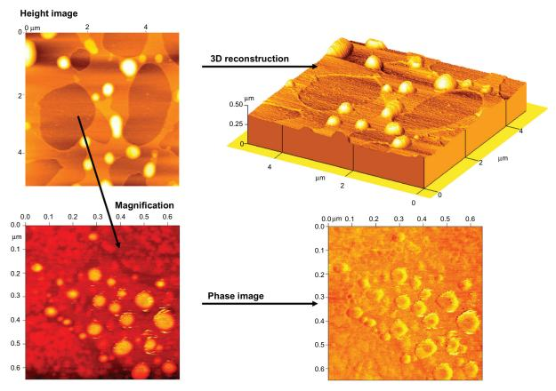
Figure 1 TM-AFM analysis (images acquired within 10–15 minutes from deposition on mica support) Abbreviations: TM-AFM, tapping mode atomic force microscopy.
