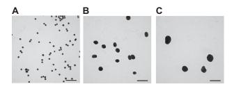
Figure I Representative transmission electron microscope images of A) 20 nm, B) 40 nm, and C) 60 nm citrate-stabilized gold nanoparticles in water. Scale bars 100 nm.
