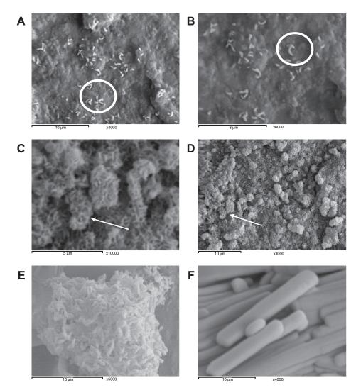
Figure I Nanoparticles (A), close up of theophylline nanoparticles (B), theophylline controlled agglomerates (C), close up of theophylline controlled agglomerates (D), aggregation of theophylline nanoparticles upon using high concentration of NaCl (E), and theophylline powder without processing (F). Note the circles that showing the mechanism of self-assembly of nanorods on a copper grid. The arrows show fluffy spherical nanorods of the controlled agglomerates.
