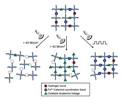
Figure 5 Designed US-induced responses of Fe3+-[PEG-Dopa]4 Hydrogels.
