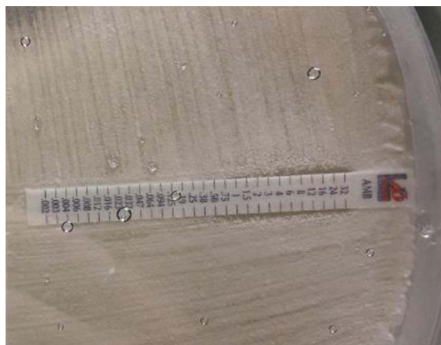
Figure 1 Amphotericin MIC test strip with Aspergillus flavus .
