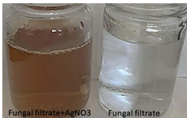
Figure 2 Biosynthesis of AgNPs indicated by color change for the reaction medium composed of 1 mM \text{AgNO}_3 and fungal filtrates after 24 h (left side) and fungal filtrate (right side).
