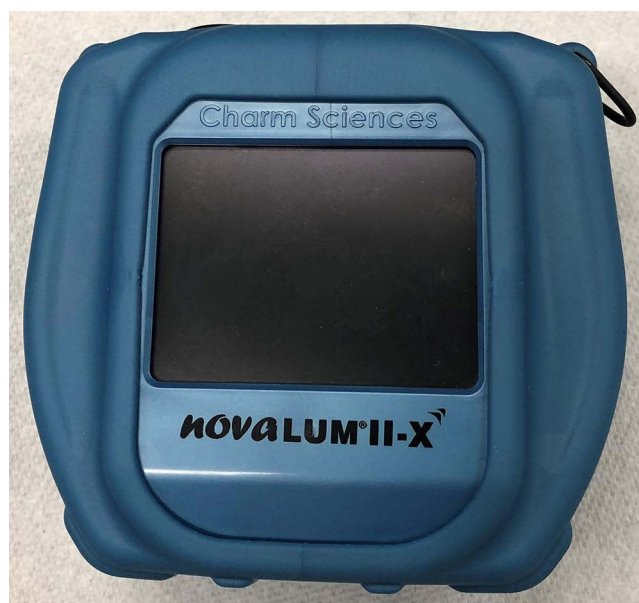
Figure 3 Charm Novalum II-X ATP biofluorescence measuring unit.
