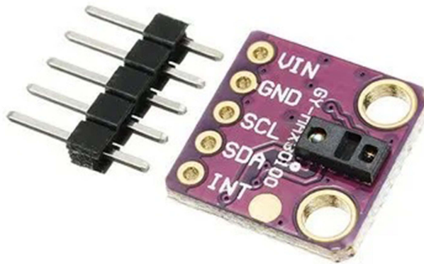
Figure 2 GY-MAX30100 pulse oximeter and heart rate sensor. Image reproduced with permission from Maxim Integrated. 22
