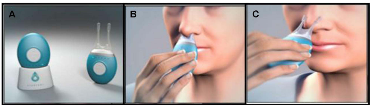
Figure 1 Intranasal neurostimulator and various application methods. (A) Intranasal neurostimulator device; (B) intranasal application; (C) extranasal application (Photos courtesy of Allergan®).
