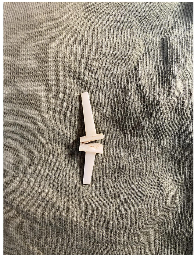
Figure 7 Typical implant fracture models in group B.
