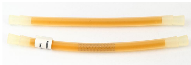
Figure 1 Image of a reference phantom (top) and a stented vessel phantom (bottom, Taxus Liberté 5/32), both filled with tracer dilution (1:100, Resovist, I'rom Pharmaceuticals, Tokyo, Japan). The stented phantom has a slightly curved shape caused by the storage of the phantoms as wound tubes. For imaging, all phantoms were straightly aligned on a dedicated phantom holder.
