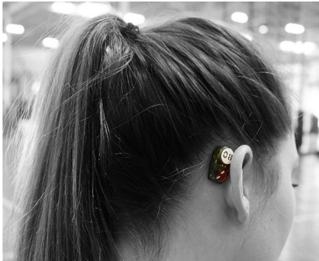
Figure 1 Phybrata sensor attached to the mastoid using an adhesive patch.
