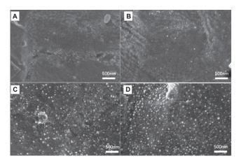
Figure I Representative SEM images of uncoated Ti A) and Se-coated Ti with low B) medium C) or high D) doses of Se nanoclusters. Note: Scale bars are 500 nm. Abbreviations: Se, selenium; SEM, standard error of mean; Ti, titanium.
