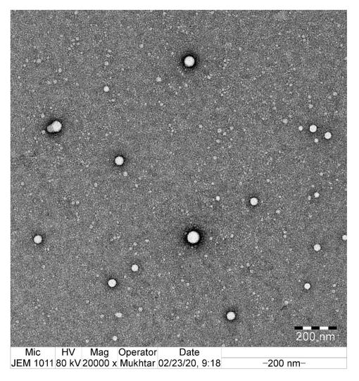
Figure 3 TEM image of optimized clarithromycin nanoparticle (CTM-CHNPopt).
