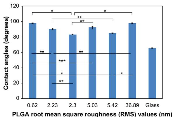
**Figure 3** dH<sub>2</sub>O static contact angles on PLGA samples. Static contact angles were obtained immediately after the deposition of a 3  $\mu$ L drop of dH<sub>2</sub>O under ambient conditions. **Notes:** Values are mean  $\pm$  SEM, n = 3. \* $P < 0.01$ , \*\* $P < 0.05$  and \*\*\* $P < 0.1$ . **Abbreviations:** dH<sub>2</sub>O, distilled water; PLGA, poly(lactic-co-glycolic) acid; SEM, standard error of the mean.
