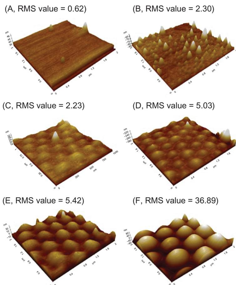
**Figure 2** AFM images and RMS values: (A–B) AFM images of PLGA surfaces created by solution evaporation with (A) 0.5 g PLGA:8 mL chloroform, (B) 0.5 g PLGA:4 mL chloroform. (C–F) AFM images of PLGA surfaces created by using templates of PS nanobeads with a diameter of (C) 190 nm, (D) 300 nm, (E) 400 nm and (F) 530 nm. **Abbreviations:** AFM, atomic force microscopy; RMS, root mean square roughness; PLGA, poly-lactic-co-glycolic acid; PS, polystyrene.
