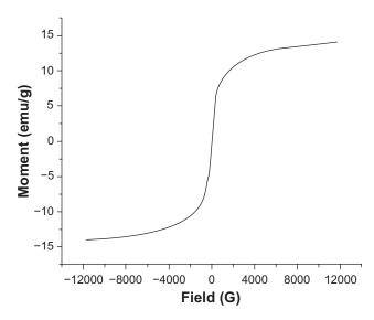
**Figure 6** Magnetization curves of IO/PVA nanoparticles as measured by VSM at room temperature. The results clearly showed superparamagnetic behavior of the nanoparticles.
