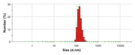
Figure 3 IO nanoparticle size distribution as measured by dynamic light scattering. **Abbrevation:** IO, iron oxide.
