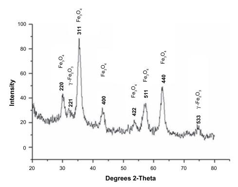
Figure 5 X-ray diffraction results of synthesized nanoparticles confirmed the existence of magnetite (Fe<sub>3</sub>O<sub>4</sub>) and maghemite γ-Fe<sub>2</sub>O<sub>3</sub>.
