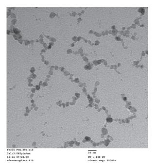
Figure 2 Transmission electron microscope images of the synthesized IO/PVA nanoparticles. Scale bar = 20 nm.
