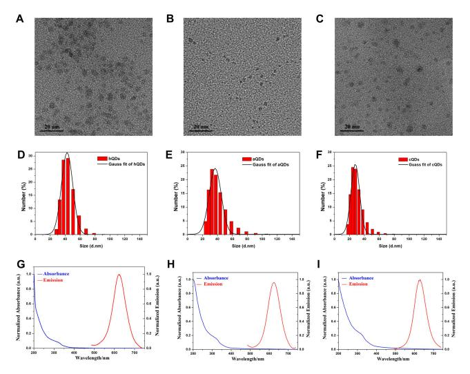
Figure I Characterization of InP/ZnS QDs with different surface modifications. (A–C) TEM image of hQDs, aQDs, and cQDs, respectively. (D–F) DLS of hQDs, aQDs and cQDs dispersed in deionized water. (G-I) Normalized absorption spectra and normalized PL spectra of hQDs, aQDs and cQDs, respectively.
