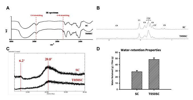
Figure I Physical characterization of mechanically nanosized sacchachitin (SC) and chemically TEMPO-oxidized sacchachitin nanofibers (T050SC). (A) FT-IR spectrum, (B) <sup>13</sup>C ssNMR, (C) X-ray powder diffraction, (D) Water retention.
