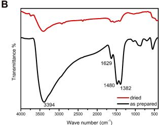
Figure 1 (A) XRD pattern of the prepared ternary nanocomposite, (B) FTIR pattern of the prepared ternary nanocomposite.
