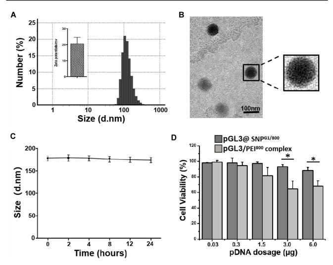
Figure 3 pGL3@SNP<sup>G1/800</sup> preparation and evaluation. (A). Hydrodynamic size distribution and zeta potential of pGL3@SNPs<sup>G1/800</sup>. (B). TEM image of pGL3@SNPs<sup>G1/800</sup>. (C). Hydrodynamic size of pGL3@SNPs<sup>G1/800</sup> in PBS buffer (pH of 7.4) at different time points. (D). Viability of Jurkat cells treated with pGL3@SNPs<sup>G1/800</sup> or pGL3/PEI<sup>800</sup> complexes at varying doses of pGL3 (\*P<0.05).
