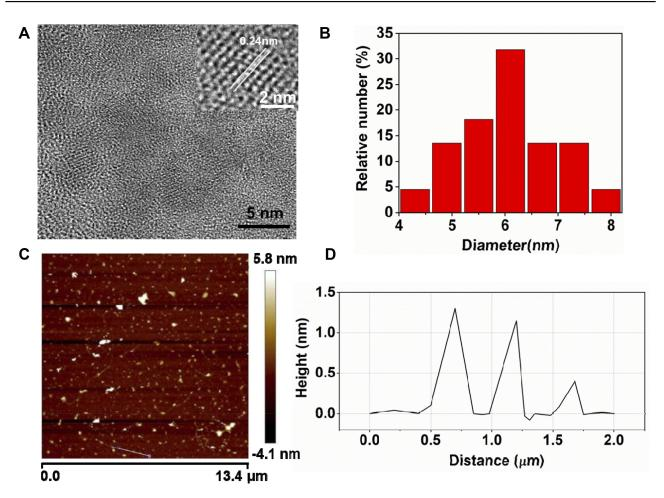
Figure I Characterizations of Mn-MoS<sub>2</sub> QDs: (A) TEM images of Mn-MoS<sub>2</sub> QDs (inset, high-resolution TEM images), (B) size distributions of Mn-MoS<sub>2</sub> QDs, (C) AFM image of Mn-MoS<sub>2</sub> QDs, and (D) size and height distributions of the MoS<sub>2</sub> QDs.
