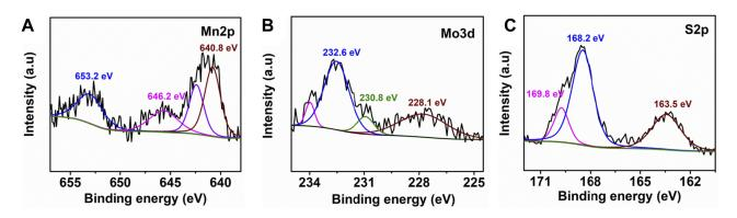
Figure 2 XPS spectra of the Mn-MoS<sub>2</sub> QDs: (A) Mn2p, (B) Mo3d, and (C) S2p.
