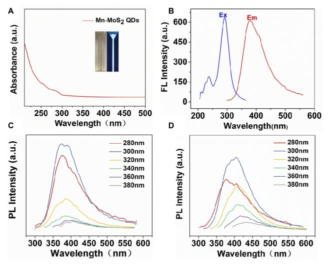
Figure 3 Optical properties of  $Mn-MoS_2$  QDs: (A) UV-vis absorption spectra of  $Mn-MoS_2$  QDs, (B) PL emission and excitation of the  $Mn-MoS_2$  QDs, (C) fluorescence emission spectra of the  $Mn-MoS_2$  QDs at different excitation wavelengths, and (D) fluorescence emission spectra of the  $Mn-MoS_2$  QDs at different excitation wavelengths.
