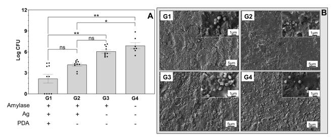
Figure 2 PDA-assisted treatment had higher bacteria killing. (A) Colony-forming units (CFU, log scale) recovered from the substrates after the treatment (data = mean ± standard error of the mean, n=5, \*p<0.05, \*\*p<0.001). (B) Representative SEM images of the sample surface after the treatments.
