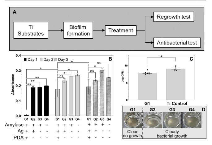
Figure 3 PDA-assisted treatment rendered the surface antimicrobial. (A): Procedure of the tests. (B): Regrowth of bacteria from treated samples monitored by OD measurement (data = mean ± standard error of the mean, n=2). (C): Significant lower log CFU on GI compared to Ti control. (data = mean ± standard error of the mean, n=3). \*p<0.05. \*\*p<0.001. (D): Photographs showing the turbidity of the broth indicating bacterial growth except for the GI group.
