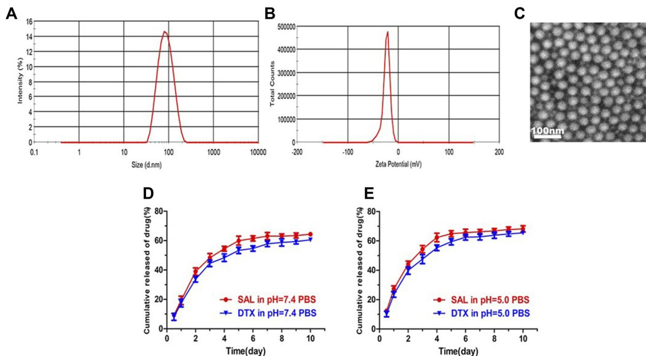
**Figure 2** Characterization of nanoparticles. Size distribution (A) and zeta potential of nanoparticles (B), as determined by dynamic light scattering. The TEM image of nanoparticles (C). Bars represent 100 nm. One representative image is shown. The cumulative release of SAL or DTX from nanoparticles at pH 7.4 (D) and 5.0 (E). Data are presented as means  $\pm$  standard deviations ( $n = 3$ ).
