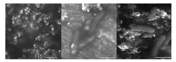
Figure 4 SEM images of (**A**) nanoparticles at 79 kx. Scale bar corresponds to 500 nm, (**B**) *E. coli* at 46.2 kx. Scale bar corresponds to 2 μm and (**C**) *E. coli* after exposure to BUF-II-PEA-magnetite nanobioconjugates at 79 kx. Scale bar corresponds to 1 μm.
