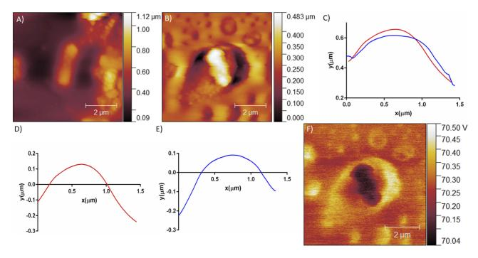
Figure 3 AFM height images of (**A**) *E. coli* (**B**) *E. coli* in the presence of BUF-II-PEA-magnetite nanobioconjugates (**C**) Height profiles of *E. coli* (red) and *E. coli* in the presence of BUF-II-PEA-magnetite nanobioconjugates (blue) (**D**) *E. coli* roughness profile for *E. coli* (red) and (**E**) *E. coli* in the presence of BUF-II-PEA-magnetite nanobioconjugates (blue) (**F**) Electrostatic force on a single bacterium after exposure to the BUF-II-PEA-magnetite nanobioconjugate.
