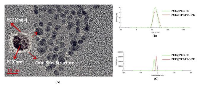
Figure 2 Characterization of PUE@TPP/PEG-PE micelles. (A) TEM photographs. (B) Size and (C) zeta potential distribution of PUE@PEG-PE and PUE@TPP-PEG-PE micelles.
