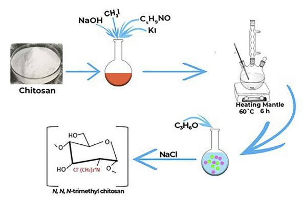
Figure I Schematic illustration of chitosan methylation for the synthesis of trimethyl chitosan polymer. **Abbreviations:** NaOH, sodium hydroxide; CH<sub>3</sub>I, Methyl iodide;  $C_5H_9NO$ , N-Methyl-2-pyrrolidone; KI, Potassium iodide;  $C_3H_6O$ , acetone; NaCl, Sodium chloride.
