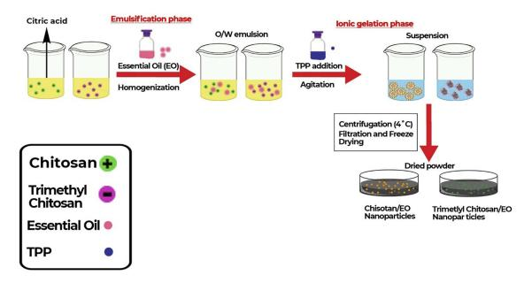
Figure 2 Process illustration for the optimised synthesis of Ocimum gratissimum essential oil-loaded chitosan and N, N, N chitosan nanoparticles. Abbreviation: TTP, tripolyphosphate.
