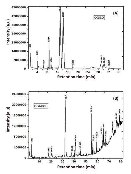
Figure 3 GC- MS chromatogram: (A) O. gratissimum essential oils and (B) methanolic extracts. Peak numbers refer to Tables I and 2, respectively.
