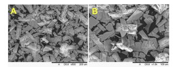
Figure 5 SEM images of Ho(acac)<sub>3</sub>×3H<sub>2</sub>O in Tabletop Microscope TM3000. Magnifications: (**A**) 500× and (**B**) 1000×. Abbreviation: SEM, scanning electron microscopy.
