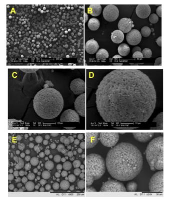
Figure 2 SEM images of PHB-HV 8%-MS in Philips XL30 Microscope (A-C) and Tabletop Microscope TM3000 (D-F). Magnifications:  $(A) 100^{\times}$ ,  $(B) 500^{\times}$ ,  $(C) 1000^{\times}$ ,  $(D) 500^{\times}$ ,  $(E) 1000^{\times}$ , and  $(F) 2000^{\times}$ .
