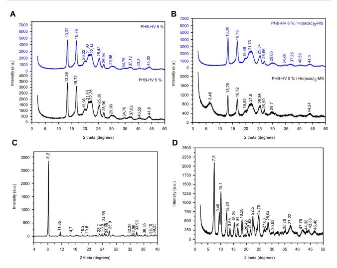
Figure 9 X-ray diffractograms of: (A) raw PHB-HV, (B) PHB-HV loaded with Ho(acac)<sub>3</sub>-MS, (C) Ho(acac)<sub>3</sub>-crystalline, and (D) Ho(acac)<sub>3</sub>-amorphous. Abbreivations: PHB-HV, poly(3-hydroxi-butyrate-co-3-hydroxy-valerate); MS, microspheres.
