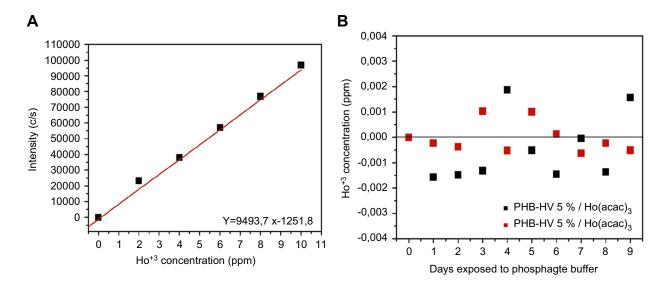
Figure II (A) Calibration curve to a standard holmium chloride solutions; (B)  $Ho^{+3}$  concentration in ppm, dosed of the microspheres solutions according to days of exposition to sodium phosphate buffer, pH 7.4.
