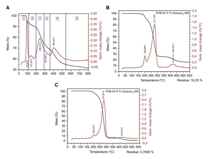
Figure 10 Thermogravimetric curves and their first derivatives obtained for: (A) raw Ho(acac)<sub>3</sub>; (B) PHB-HV 5%/Ho(acac)<sub>3</sub>-MS; (C) PHB-HV 8%/Ho(acac)<sub>3</sub>-MS. Abbreivations: PHB-HV, poly(3-hydroxi-butyrate-co-3-hydroxy-valerate); MS, microspheres.
