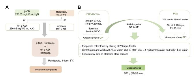
Scheme I Schematic illustration of the synthesis of the inclusion compounds in  $\beta$ -cyclodextrins and of the microspheres with PHB-HB. (A) Preparation of the  $\beta$ -cyclodextrin-holmium acetylacetonate and the hydroxyl-propyl- $\beta$ -cyclodextrin inclusion complexes. (B) Emulsification process to prepare PHB-HV 5% microspheres. \*The PHB-HV 8% microspheres were prepared following the same scheme.
