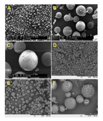
Figure I SEM images of PHB-HV 5%-MS in: Philips XL30 Microscope (A-C) and Tabletop Microscope TM3000 (D-F). Magnifications: (A) 100×, (B) 500×, (C) 1000×, (D) 200×, (E) 500×, and (F) 2000×.
