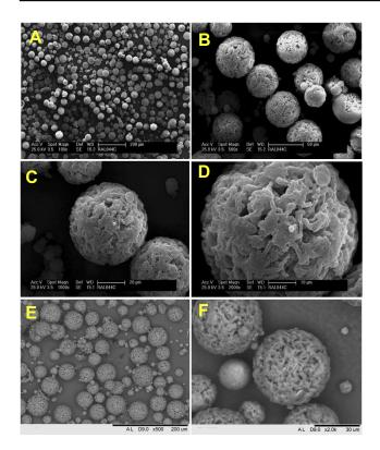
Figure 4 SEM images of PHB-HV 8%/Ho(acac)<sub>3</sub>-MS in Philips XL30 Microscope (A-D) and Tabletop Microscope TM3000 (E-F). Magnifications: (A) 100×, (B) 500×, (C) 1000×, (D) 2000×, (E) 500×, and (F) 2000×.
