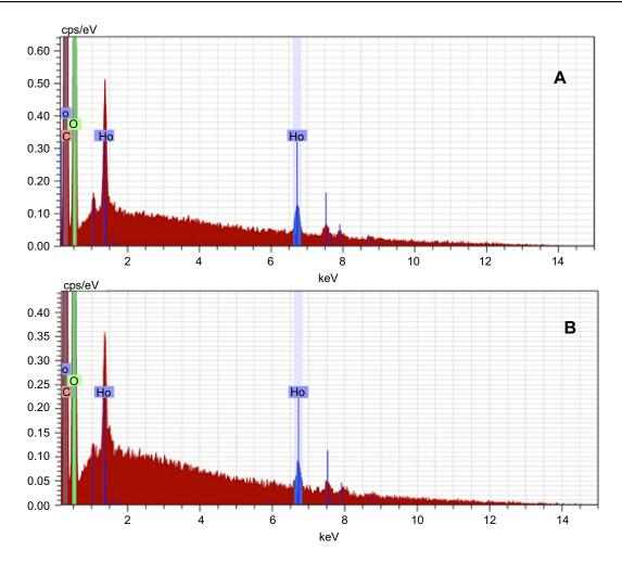
Figure 6 The EDS spectra of (A) PHB-HV 5%/Ho(acac)<sub>3</sub>-MS; and (B) PHB-HV8%/Ho(acac)<sub>3</sub>-MS, both acquired in Tabletop Microscope TM3000. Abbreviatons: EDS, energy-disperSive x-ray; PHB-HV, poly(3-hydroxi-nutyrate-co-3-hydroxy-valerate); MS, microspheres.
