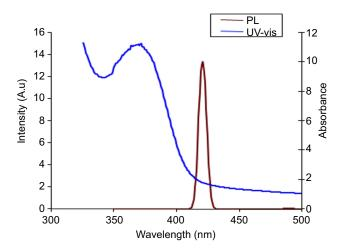
Figure 2 UV-vis and PL spectra of AgNPs@PPE. Abbreviations: PL, photoluminescence; UV-vis, ultraviolet-vis spectrophotometry.
