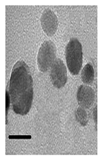
Figure 3 TEM image of the AgNPs@PPE (scale bar is 50 nm). Abbreviation: TEM, transmission electron microscopy.
