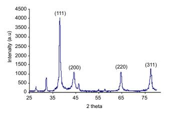
**Figure I** XRD pattern of AgNPs@PPE. **Abbreviation:** XRD, X-ray diffraction.
