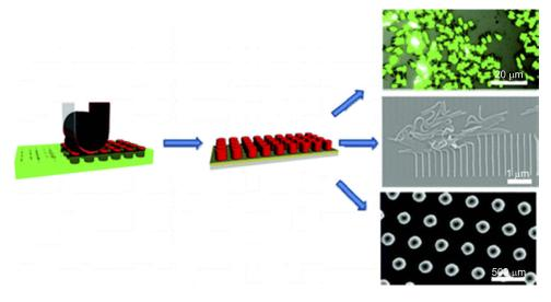
Figure 6 Scheme showing the imprint lithography method used to fabricate different shapes of nanoparticles. Note: Reprinted with permission from Merkel TJ, Herlihy KP, Nunes J, Orgel RM, Rolland JP, DeSimone JM. Scalable, shape-specific, top-down fabrication methods for the synthesis of engineered colloidal particles. *Langmuir.* 2010;26(16):13086–13096. Copyright © 2010 American Chemical Society.<sup>37</sup>
