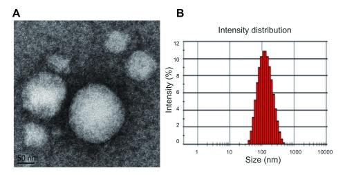
Figure 2 The characterization of (DSPE)-PEG<sub>2000</sub>-FA-LPs/CUR.**Notes:** (**A**) The transmission electron microscope images; (**B**) the size distribution. **Abbreviations:** DSPE, Distearoyl-L-a-phosphatidylethanolamine; CUR, Curcumin FA, folic acid; LP, liposome.
