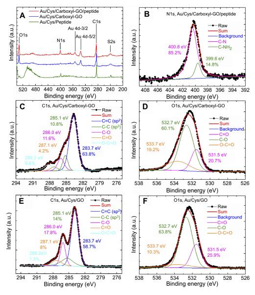
Figure 3 High resolution XPS spectra of the carboxyl-GO and GO films. (A) Survey scan XPS spectra of the different sensing chips. (B) NIs region for the as-formed carboxyl-GO/peptide chip. (C) CIs and (D) OIs regions for the as-formed carboxyl-GO chip. (E) CIs and (F) OIs regions for the as-formed GO film.
