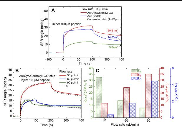
Figure 5 (A) The injection of peptides at a flow rate of 30 µL/min showing the three different SPR chip binding reactions. (B) The injection of peptides at different flow rates showing the carboxyl-GO ship binding reaction. (C) The binding kinetic constants at different flow rates in association and dissociation analyses.
