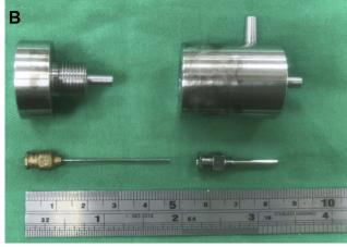
**Figure I (A)** Schematic of the experimental setup to co-axially electrospin the sheath-core-structured nanofibers; **(B)** photo of the co-axial nozzle and needles used for the experiments.
