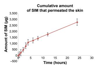
Figure 6 Percentage of SIM permeated through the rat skin from the prepared nanosized hydrogel. Abbreviation: SIM, simvastatin.
