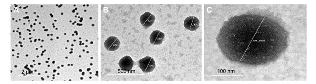
Figure 3 TEM images of F20 at (A) 2  $\mu$ m resolution, (B) 500 nm resolution showing the particle size range from 177.6 to 200 nm, and (C) 100 nm (the drug distributed as white spots on the particle surface).
