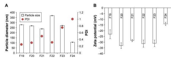
Figure 2 (A) Particle size and PDI of the prepared formulae. (B) Zeta potential for the prepared formulae. Abbreviation: PDI, polydispersity index.
