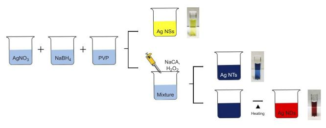
Figure 1 Schematic illustration for synthesis of the Ag NPs with different shapes.
