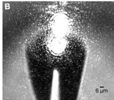
Figure I Bright-field microscopic images of the fabricated polymeric tip on the top of a single mode optical fiber dropped into a solution of distilled water.
