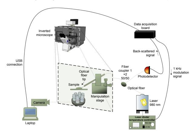
Figure 2 Scheme of the optical setup used to manipulate the fiber tool with the micro-lens on its extremity and acquire the back-scattered signal for nanoparticles detection in acuse us media
