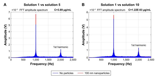
Figure 5 Single-sided amplitude spectrum of the Fast Fourier Transform (FFT) of filtered back-scattered signal portions of 60 seconds before being z-scored and acquired using distilled water and 100 nm nanoparticles solutions in concentrations of (**A**) 3.89 μg/mL and (**B**) 1.22E-03 μg/mL.
