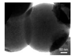
Figure SI TEM image of BG microspheres without hollow structure. Abbreviations: BG, bioglass; TEM, transmission electron microscopy.
