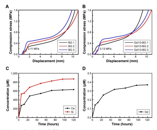
Figure S2 Mechanical property and ion release kinetics of scaffolds. Notes: Compression strengths of different samples: (A) BG scaffolds; (B) Gd1/3-BG scaffolds. Ion release performances of Gd1/3-BG scaffolds: (C) Ca and Si ions; (D) Gd ions. Abbreviations: BG, bioglass; Gd, gadolinium.
