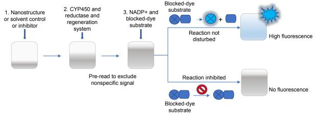
Figure I A schematic representation of Baculosomes®-based enzymatic test for CYP catalytic activity measurements. Notes: The enzymatic reaction is initiated by the addition of a mix of NADP+ and the proper substrate. During the reaction, the dye (blue circle) is being released from the substrate (blue rectangle), forming fluorescent product. Details in the main text of the "Materials and methods" section.
