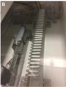
Figure 1 (A) Smoke-exposure system with one exposure chamber. (B) Cigarette feeder and pumping system (Candela Constructions®).
