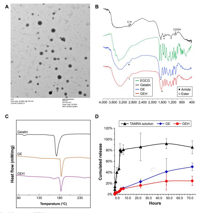
Figure 2 Characterization of EGCG-loaded nanoparticles. Notes: (A) TEM morphology of GEH using an HA concentration of 62.5  $\mu$ g/mL. (B) FTIR spectra, (C) DSC thermography, and (D) release patterns of variant formulations.
