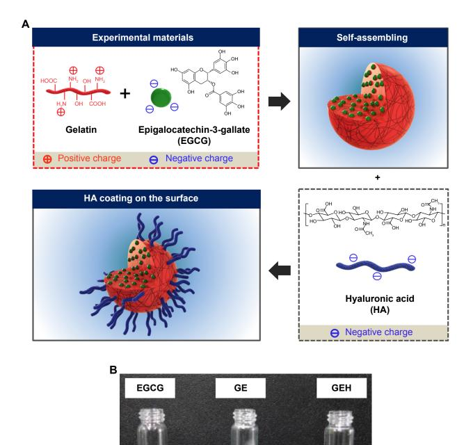
Figure 1 Schematic representations of (A) self-assembled GE and GEH NP formation and (B) photograph of these colloidal solutions.
