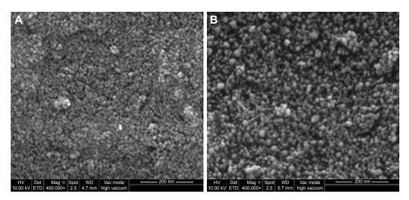
Figure 5 Surface morphology of magnetite nanoparticles with 0.5% and 3% (w/v) honey (A) and (B), respectively.
