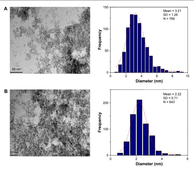
Figure 4 TEM images and histograms of particle size distribution for 0.5% and 3% (w/v) honey/Fe<sub>3</sub>O<sub>4</sub>-NPs. (**A**) and (**B**): 0.5% and 3% (w/v), respectively. **Abbreviations:** Fe<sub>3</sub>O<sub>4</sub>-NPs, magnetite nanoparticles; TEM, transmission electron microscopy.
