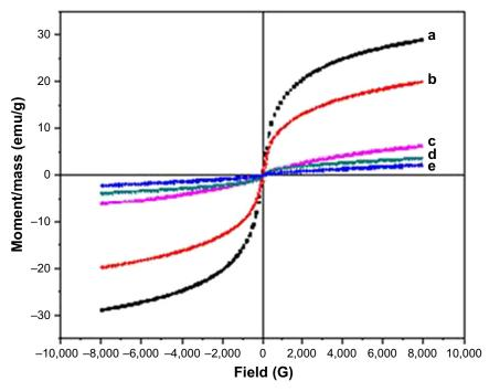
Figure 7 VSM of pure  $Fe_3O_4$  (a) and  $Fe_3O_4$ -NPs with 0.5, I, 3 and 5% (w/v) honey (b–e, respectively). Abbreviations:  $Fe_3O_4$ -NPs, magnetite nanoparticles; VSM, vibrating sample magnetometry.
