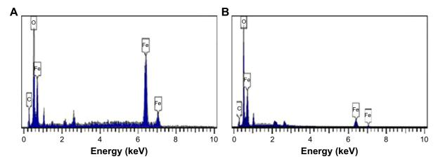
Figure 6 EDX spectroscopy of  $Fe_3O_4$ -NPs with 0.5% and 3% (w/v) honey, (**A**) and (**B**), respectively. Abbreviations: EDX, energy-dispersive X-ray;  $Fe_3O_4$ -NPs, magnetite nanoparticles.
