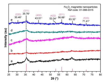
Figure 2 Powder X-ray diffraction patterns of  $Fe_3O_4$ -NPs without (a) and with different concentrations of honey (0.5, I, 3, and 5% [w/v]) (b–e), respectively. Abbreviations:  $Fe_3O_4$ -NPs, magnetite nanoparticles; ref, reference.
