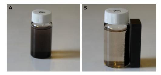
Figure I The 0.5% (w/v) honey/magnetite nanoparticles suspension without (A) and with (B) a magnetic field.
