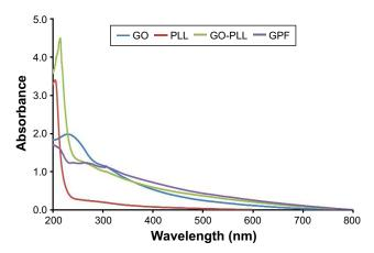
Figure SI The UV-vis spectra of GO, PLL, GO-PLL, and GPF. Abbreviations: GO, graphene oxide; GPF, graphene oxide-poly-L-lysine hydrobromide/folic acid; PLL, poly-L-lysine hydrobromide; UV-vis, UV-visible.
