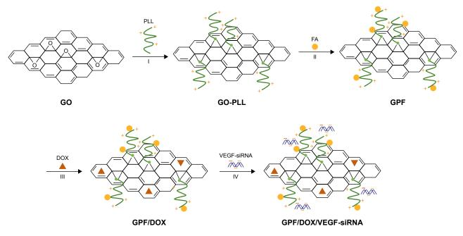
Scheme I Scheme for GPF and GPF/DOX/VEGF-siRNA preparation. (I) KOH, 70°C, 24 hours, DI water. (II) Room temperature, 24 hours. (III) Stirred at room temperature, without light, 12 hours, DI water. (IV) Incubation at 37°C, 30 minutes, DEPC water.
