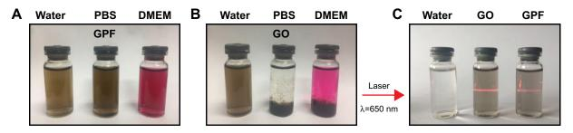
Figure 4 The dispersibility and stability of GPF (A), GO (B), and the Tyndall effect of GO and GPF (C). Abbreviations: DMEM, Dulbecco's Modified Eagle's Medium; GO, graphene oxide; GPF, GO-poly-L-lysine hydrobromide/folic acid.
