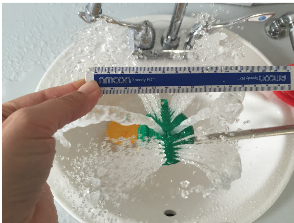
Figure 4 The water flow of an eye wash station with diverging water flow. This model includes a face wash flow of water above and below the eyes. The distance between the peaks of water flow are approximately 110 mm apart.
