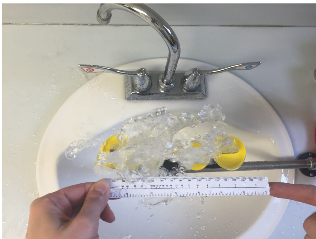
Figure 5 The water flow of an eye wash station with converging water flow. The two streams of water form one large plateau of water that will accommodate people with an inter-pupillary distance of 120 mm or less.
