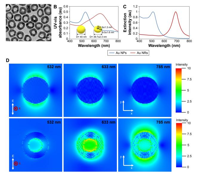
Figure I (A) Transmission electron microscope micrographs of Au NRs. (B) UV-vis absorption spectra of Au NPs and Au NRs. (C) Simulated extinction spectra of Au NPs and Au NRs through DDA calculation. (D) DDA simulated electric field intensity distribution of Au NPs (upper row) and Au NRs (lower row) at 532 nm, 633 nm, and 785 nm wavelength, respectively.
