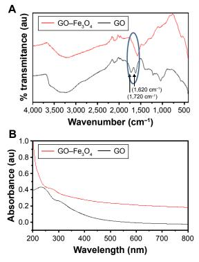
**Figure I** (**A**) FTIR spectra of GO–Fe<sub>3</sub>O<sub>4</sub> nanocomposites and of pure GO. The circle area denotes the removal of IR bands in GO at (1720 cm<sup>-1</sup>), (1620 cm<sup>-1</sup>) on the formation of GO–Fe<sub>3</sub>O<sub>4</sub>. (**B**) UV–visible absorption studies of GO and GO–Fe<sub>3</sub>O<sub>4</sub> nanocomposites.
