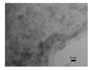
Figure 2 Transmission electron microscopy image of GO-Fe<sub>3</sub>O<sub>4</sub> nanocomposites.
