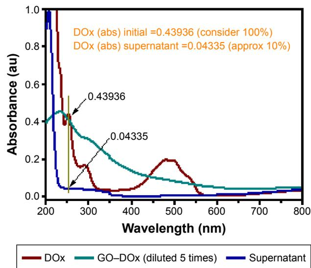
**Figure 3** Percent drug (DOx) loaded onto a GO-DOx conjugate. **Abbreviations:** au, arbitrary unit; DOx, doxorubicin; GO, graphene oxide.
