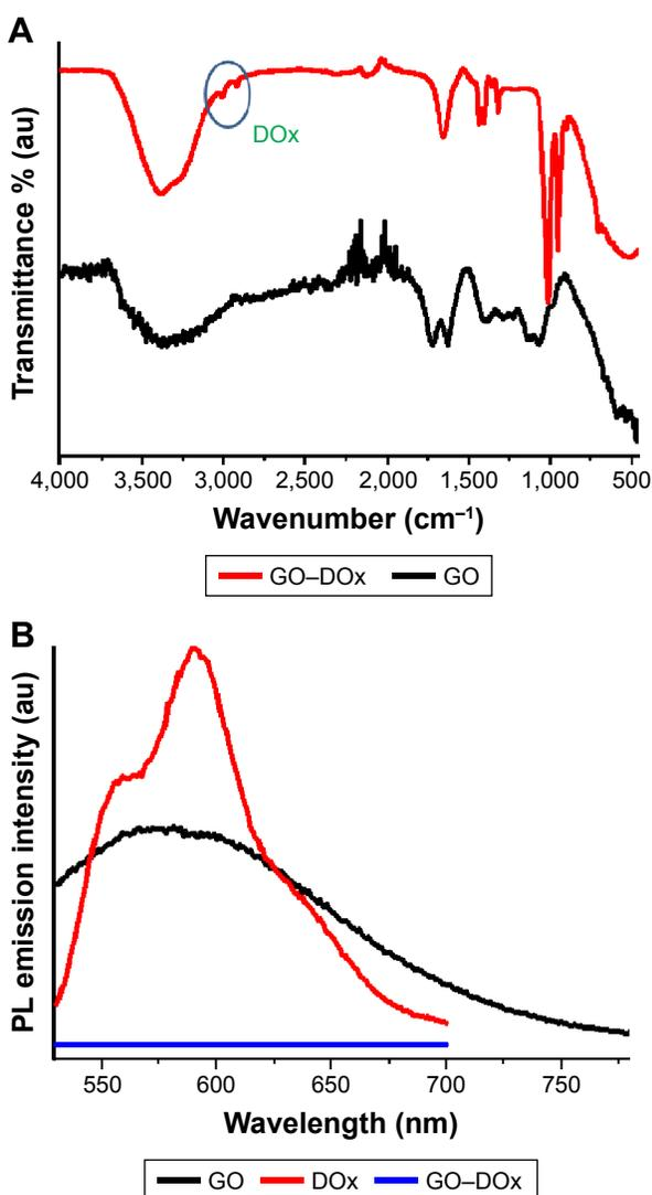
**Figure 2** (A) FT-IR spectra showing both GO and GO-DOx conjugate and (B) photoluminescence emission spectra of GO, DOx, and GO-DOx conjugate. **Abbreviations:** au, arbitrary unit; DOx, doxorubicin; FT-IR, Fourier transform infrared spectroscopy; GO, graphene oxide; PL, photoluminescence.
