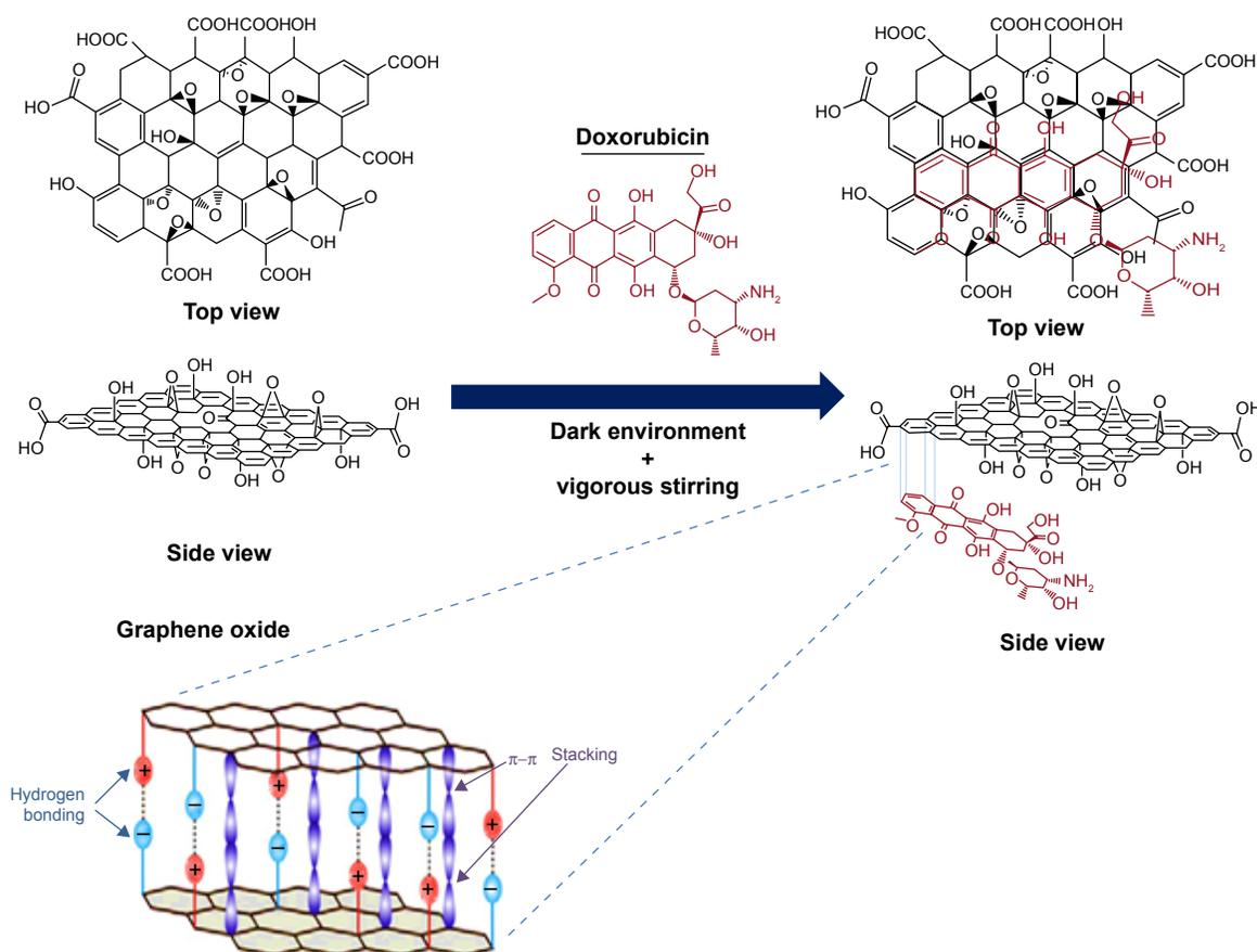
**Figure 1** Schematic representation for a graphene oxide–doxorubicin conjugation.
