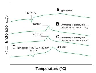
Figure 4 Differential scanning calorimetry thermogram of (A) glimepiride, (B) Eudragit® (Ammonio Methacrylate Copolymer Ph Eur) RL 100, (C) Eudragit® (Ammonio Methacrylate Copolymer Ph Eur) RS 100, and (D) physical mixture.
