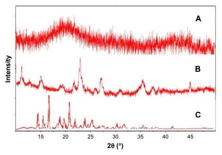
Figure 3 X-ray diffractograms of (A) glimepiride loaded polymeric patches, (B) physical mixture, glimepiride, Eudragit® (Ammonio Methacrylate Copolymer Ph Eur RL 100, and (C) pure glimepiride.
