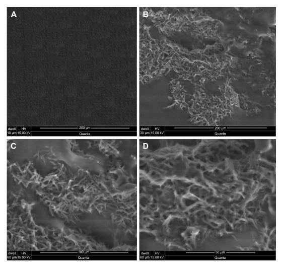
Figure 2 Scanning electron microscopy micrographs (A) before drug release at 200  $\mu$ m, (B) after drug release at 200  $\mu$ m, (C) after drug release at 100  $\mu$ m, (D) after drug release at 50  $\mu$ m.
