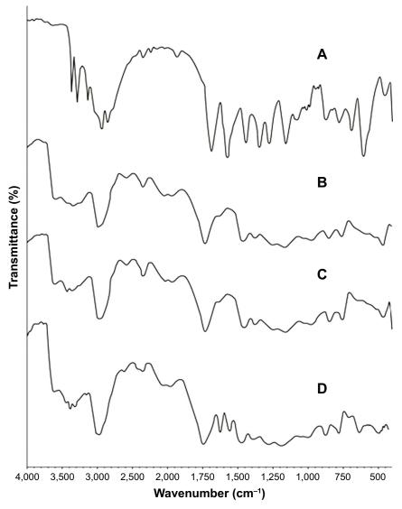
Figure I FTIR spectra of (A) Glimepiride, (B) Eudragit® (Ammonio Methacrylate Copolymer Ph Eur) RL 100, (C) Ammonio Methacrylate Copolymer Ph Eur RS 100, (D) physical mixture of polymers plus drug.
