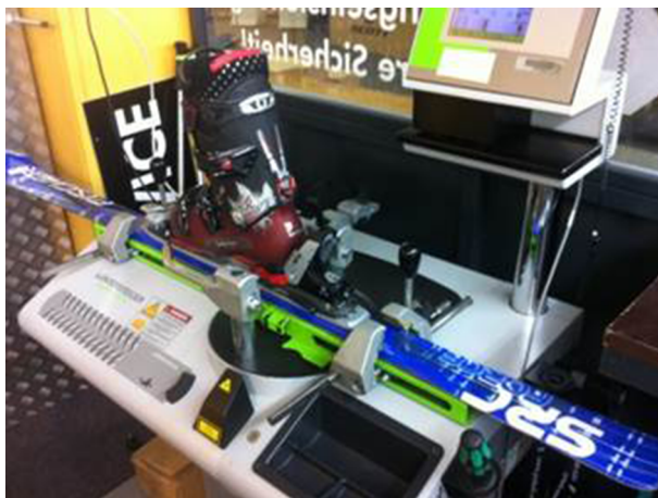
Figure 1 Wintersteiger Speedtronic – ski binding adjustment system.
