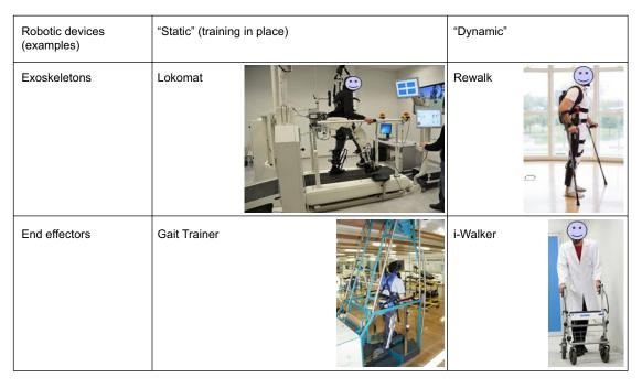
Figure 3 Examples of robotic devices with different approaches.
